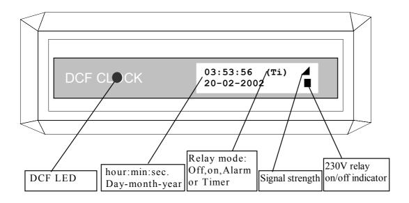
As soon as the internal time is synchronised with the DCF signal the clock will show Time, day, month, year, relay mode, signal strength and relay position.
